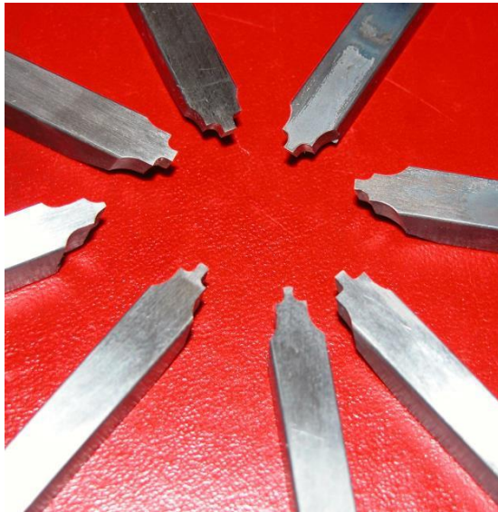
Variety of custom single point cutters I've machined the JK way
